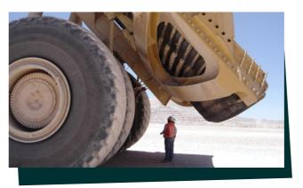
Duratray's Smart Tray (ST) is the most advanced dump tray for mining and construction trucks. The ST can monitor its condition (structural and wear) automatically and report to the user online and in real time.
