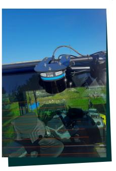
BOMAG Emergency Brake Assist is a technology designed for road construction machines that prevents collisions while protecting the hot asphalt surface from damage.
